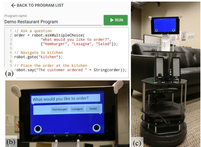
Figure 2: (a) The browser-based CodeIt interface showing a sample program, (b) the robot’s screen during the operation of the sample program, (c) the Turtlebot.
