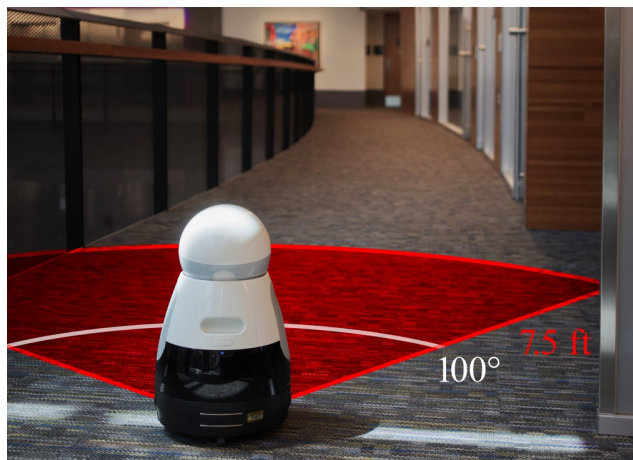
Fig. 1. Kuri in the halls of our academic building. Kuri is an expressive and engaging robot with low sensing and computation capabilities. Its lidar can only see up to 7.5 ft, insufficient to localize in long, wide hallways. Further, a significant portion of its compute gets used by localization algorithms. Motivated by these limited capabilities, in this paper we describe a system for “wandering” that enabled Kuri to traverse our large hallways for four days.
