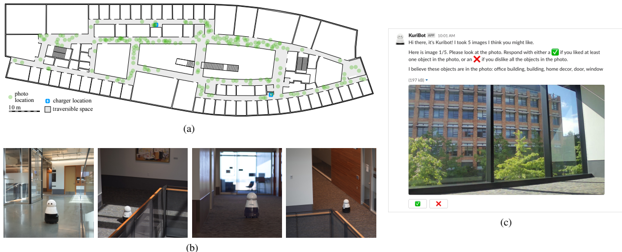
Fig. 4. (a) Kuri’s movement around the floor plan of the building. Each dot represents a location Kuri was in when it took a picture, as annotated by researchers for a random 20% of the pictures it took. (b) Photos of Kuri as it wandered the environment. The environment contains materials that are difficult to perceive with depth sensors, like glass, chrome-finish metal, and black chain-link banisters. Large windows also varied the lighting, which impacts vision-based navigation approaches. (c) An example chatbot prompt from the deployment where the robot asked a user whether they like an image it took.
