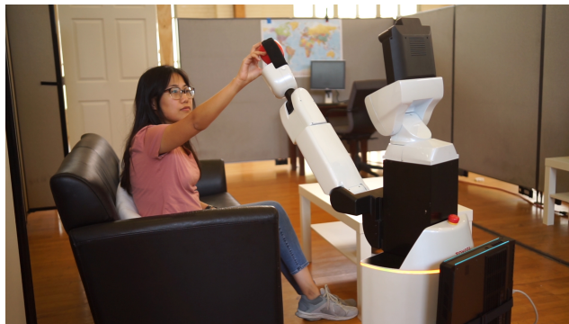
Figure 1: A Toyota Human Support Robot, representative of typical GPSRs, handing an apple to a user in a mock home environment.
