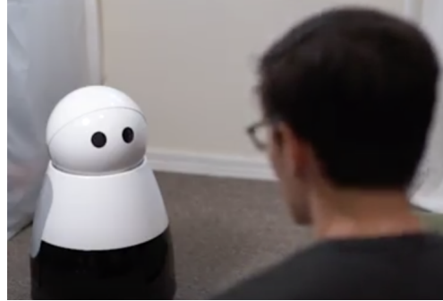
Figure 6: While the user study employed a virtual robot to adapt to the COVID-19 pandemic, we also demonstrate that our method can be deployed on a physical Mayfield Kuri robot.
