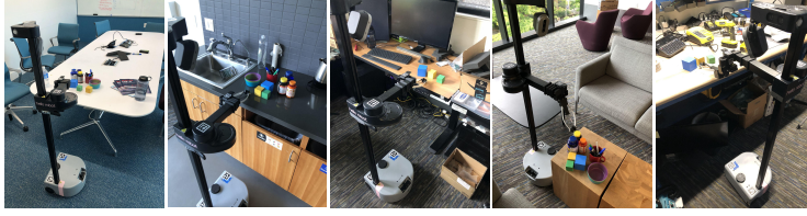
Figure 3: We evaluate SHOWTELL using a Stretch RE2 robot to perform 16 real world manipulation tasks across 5 visually distinct environments including a conference room, a kitchen, a classroom, an office lounge, and a cluttered workbench. We show that this approach is effective for teaching manipulation tasks requiring high level logic such as conditions, iteration, and segmentation.
