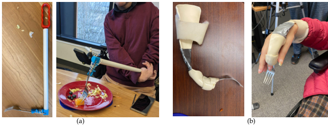
Fig. 14. (a) P3’s custom 3D-printed self-feeding tool for grasping onto and maneuvering a fork. (b) P5’s self-feeding tool for strapping a fork to her hand.
